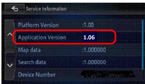
If the displayed Application Version is **1.06** or higher, then your product is equipped with the latest version and there is no need for any upgrade. If the Application Version number is lower than **1.06**, it is necessary to update the firmware. Please continue to Step B.
