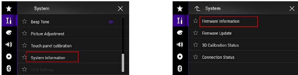
5. After the "Firmware Information" screen appears, check the firmware version number. If the firmware version is **1.15** or higher, it is not necessary to update the firmware. If the version number is lower than **1.15**, it is necessary to update the firmware. Please continue to Step B. **If the firmware version starts with 8 you have a Camper Van model and you should download a different firmware update file.**
