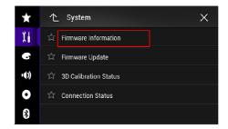
5. After the "Firmware Information" screen appears, check the firmware version number. If the firmware version is **1.21** or higher, it is not necessary to update the firmware. If the version number is lower than **1.21**, it is necessary to update the firmware. Please continue to Step B. If the firmware version starts with 8 you have a Camper Van model and you should download a different firmware update file.
