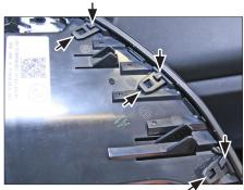
9. Remove air vents carefully (double clipped /see arrows) and air vent trim frames from OEM panel.
