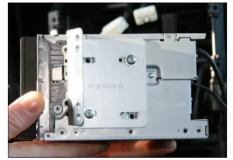
3. Attach mounting brackets to Pioneer head unit
