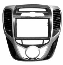
6. Mount new Double DIN facia plate to OEM center panel (see arrow) with OEM screws
