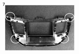
7 Insert the metal clips as shown in a photo.
