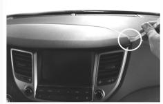
1 Remove the odometer cover frame.
