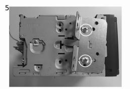
5 Take both left and right brackets and mount them on the aftermarket head unit, each one by using the supplied screws. See the picture for a correct positiong of the screws.
