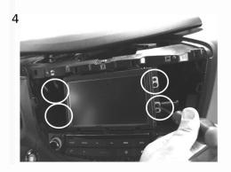
4 Remove the OEM head unit by unscrewing the circled screws (pay attention to save them them) and disconnect all cables.
