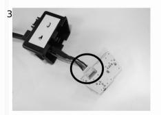
3 Take the supplied PCB, pass the cable through the aux-in hole and connect it to the circled connector.
