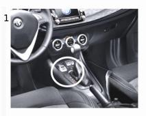
1 The USB interface is located in the circled position.
