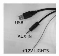
6 Plug the connector of the harness and do all connections on radio side. Insert the USB and 3,5 mm Jack replacement panel into the hole left by the OEM part.
