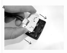
4 Slide the PCB into the front plastic part and check that the sockets are correctly positioned respect to the apertures (Jack and USB) of the plastic. Please apply some pressure so that the PCB and the plastic cover touch each other.
