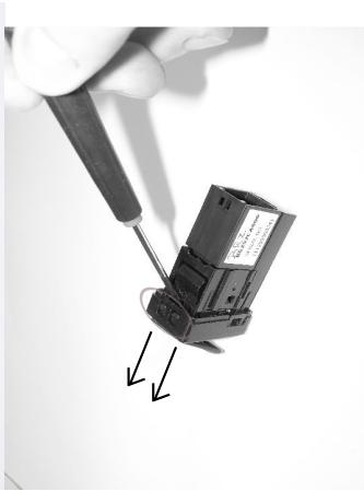
Take the front plastic removed in the previous step and mount it on the new interface. Make all the connections and replace in the car housing.
