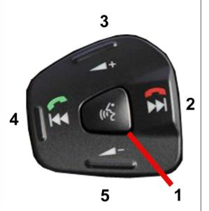
Single Press (Button 1) switches display on . Press & Hold **Speech Button** (button 1) for 2 seconds this will enable menu mode option.
