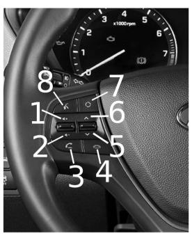
The steering wheel buttons perform the following functions (if supported by the radio and vehicle):
