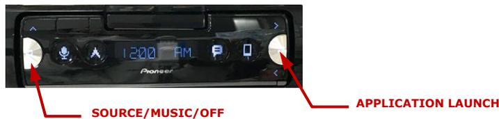
3. Press and hold the Application launch button, to display the "Initial" menu. then press to confirm.
