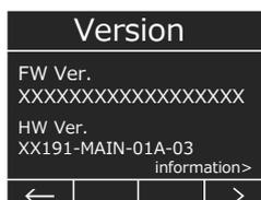
4. If the firmware version is **20220804\_1.3.0\_EW\_B** or higher, it is not necessary to update the firmware. If the version number is lower than **20220804\_1.3.0\_EW\_B**, it is necessary to update the firmware. Please continue to Step B.
