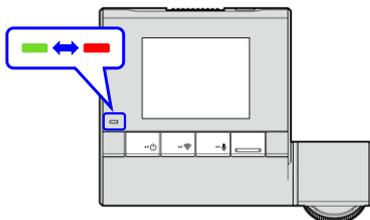
7. The update is complete when the system indicator stops flashing and the Pioneer logo appears on the screen. Next the system indicator is solid green and the recording screen appears.
